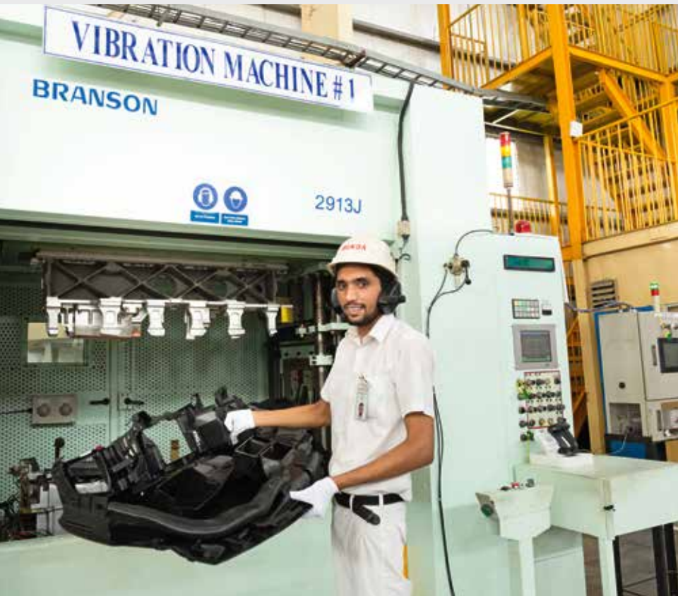
SRS Air Bag System Assembly & Seamless Welding and Vibration of Instrument Panel - PO Injection Department
