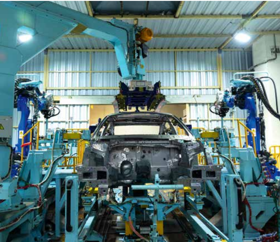
Roof Laser Brazing Process – Welding Department
