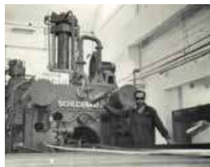
The Schloemann Press for processing aluminium cable installed
