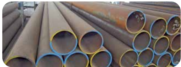
Crescent Steel procures and processes HR Coils that pass quality testing, to manufacture steel line pipes
