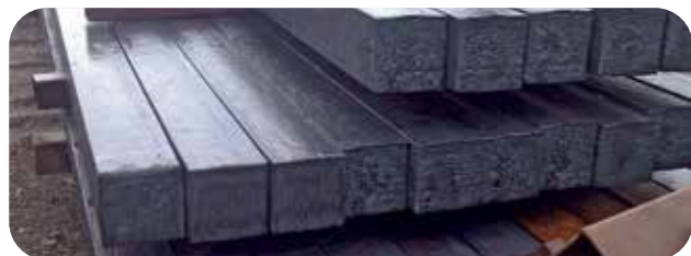
Billets are produced through a steel melting and ladle refining process. These billets are sold to rerolling mills and converted to rebar
