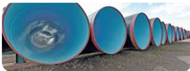
External and/or internal coating is applied to bare pipes and pipes are tested for quality.
