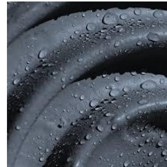
Typical transmission line disc insulator after coating
