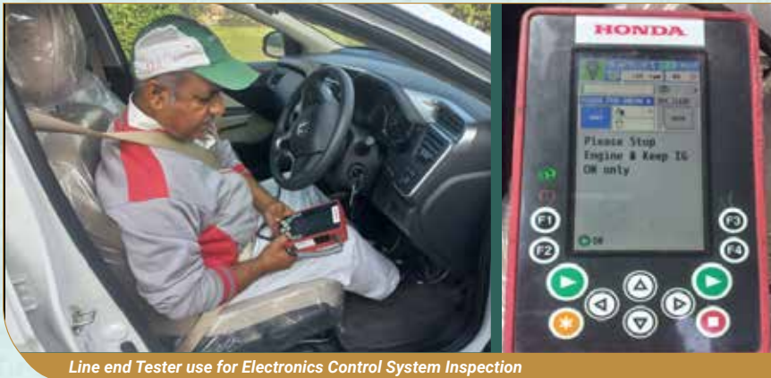
Line end Tester use for Electronics Control System Inspection
