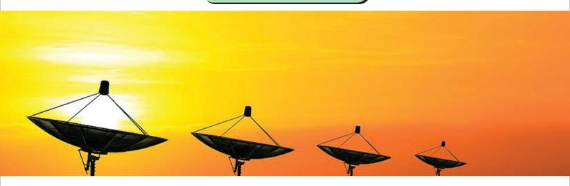
**VSAT** (Very Small Aperture Terminal) is a sophisticated communications technology that allows for the use of small fixed satellite antennas to provide highly reliable communication between a central hub and almost any number of geographically dispersed sites.
