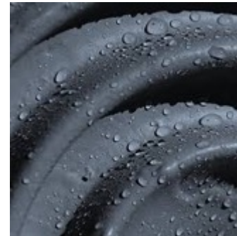
Typical transmission line disc insulator after coating
