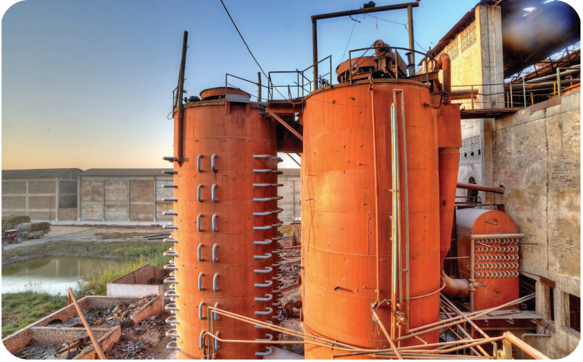
Vertical process vessels forming part of Sugar clarification & refining operation.
