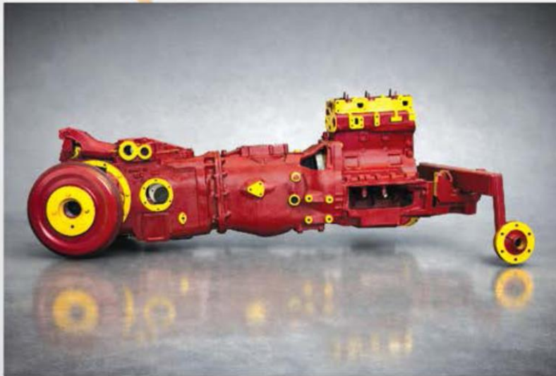
MF-240 Tractor Chassis Made from BCL Castings
