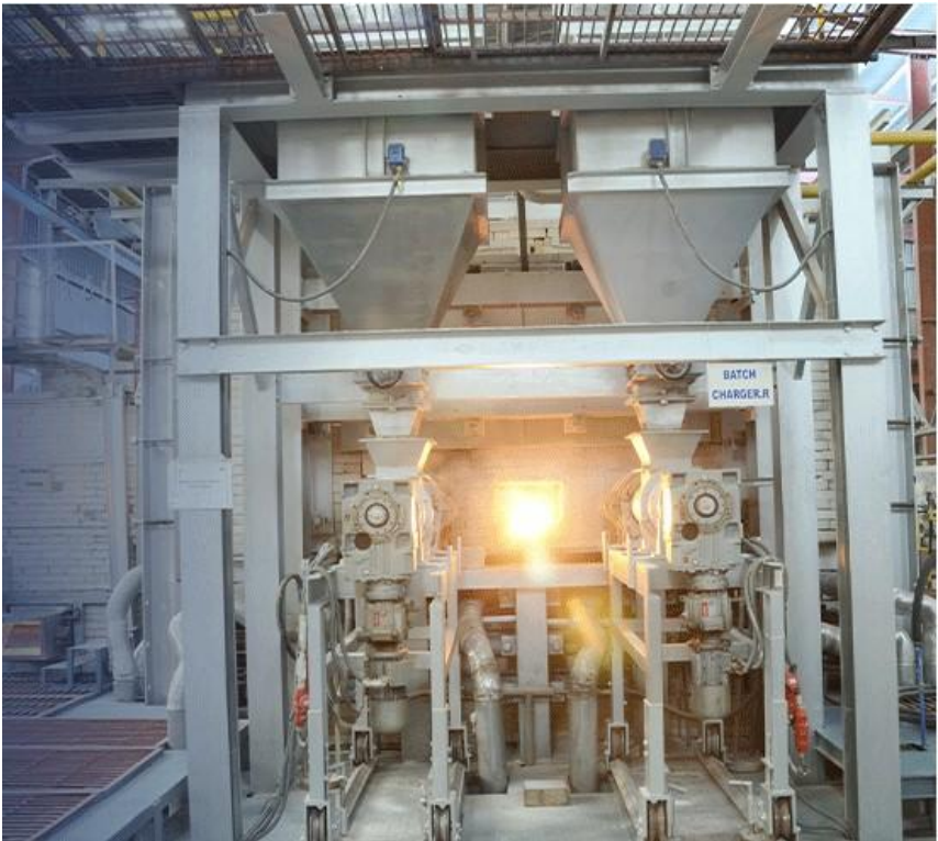
Borosilicate glass-melting furnace at the plant, 52-km Lahore–Multan Road, Phool Nagar, District Kasur
