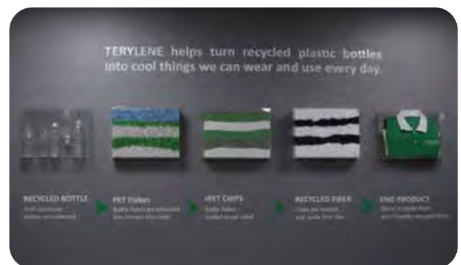
LCI's eco-friendly initiative, transforming used PET bottles into polyester fiber for a circular economy.
