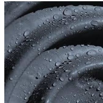
Typical transmission line disc insulator after coating
